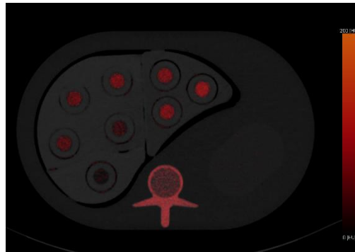
Figure 4.10 The material selective(iodine) image were reconstructed using Liver VNC application profile on Syngo.Via software.
