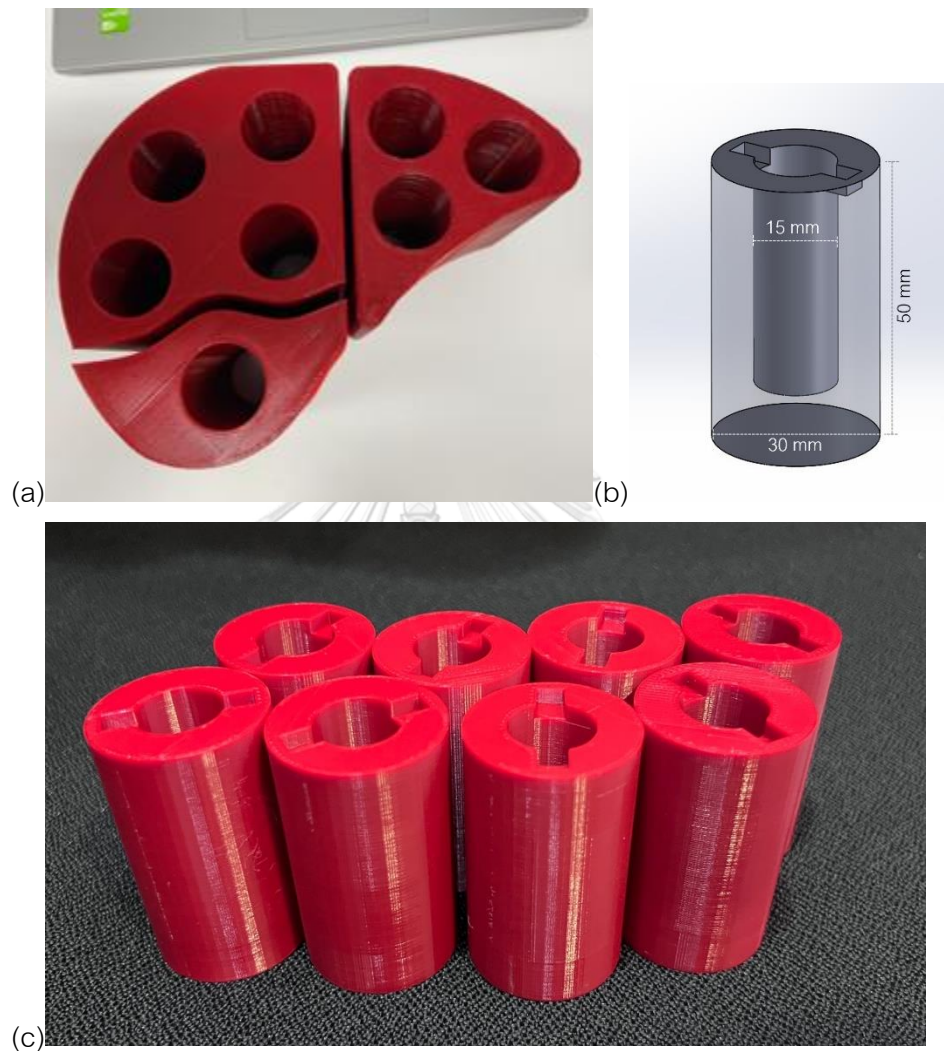
Figure 4.7 The liver phantom was constructed as 3 separated small parts (a) each part consists of the empty holes for inserted removable cylindrical container with simulated liver nodule of 15 mm diameter inserted (c).
