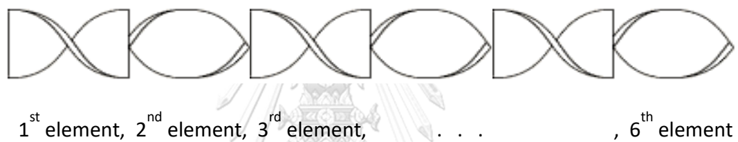
Figure C.1 The geometry of Static Mixer Elements (adapted from Noritake®)
