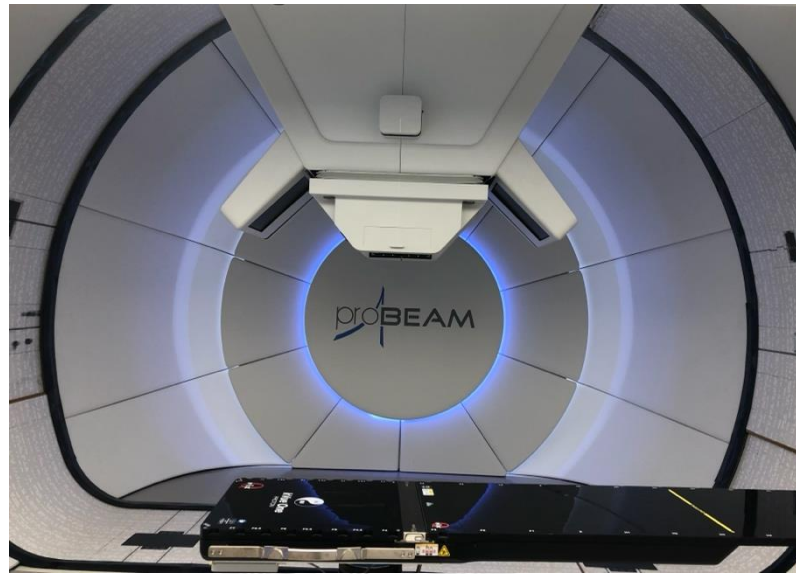
Figure 3.3 The Varian ProBeam™ Compact spot scanning system.
