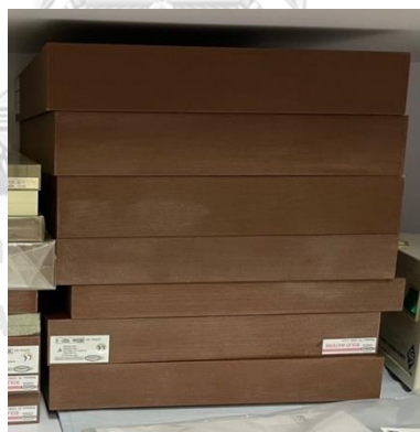
Figure 3.5 Solid water phantom.
