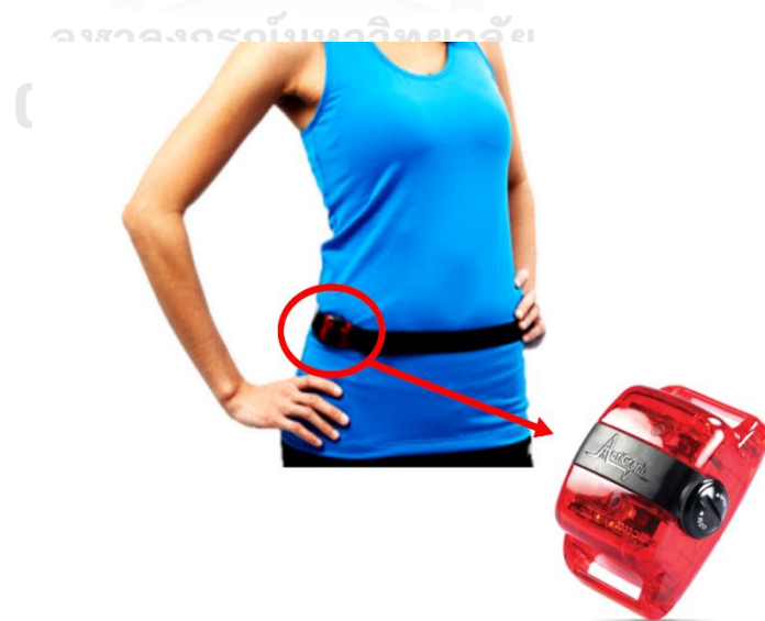
Figure 11, The illustration of GT3X+ accelerometer sensor wearing
