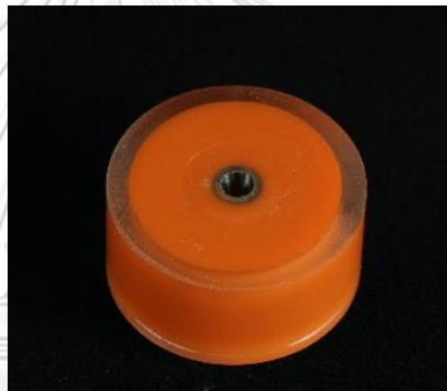
Figure 2 The implant fixture embedded in epoxy resin
