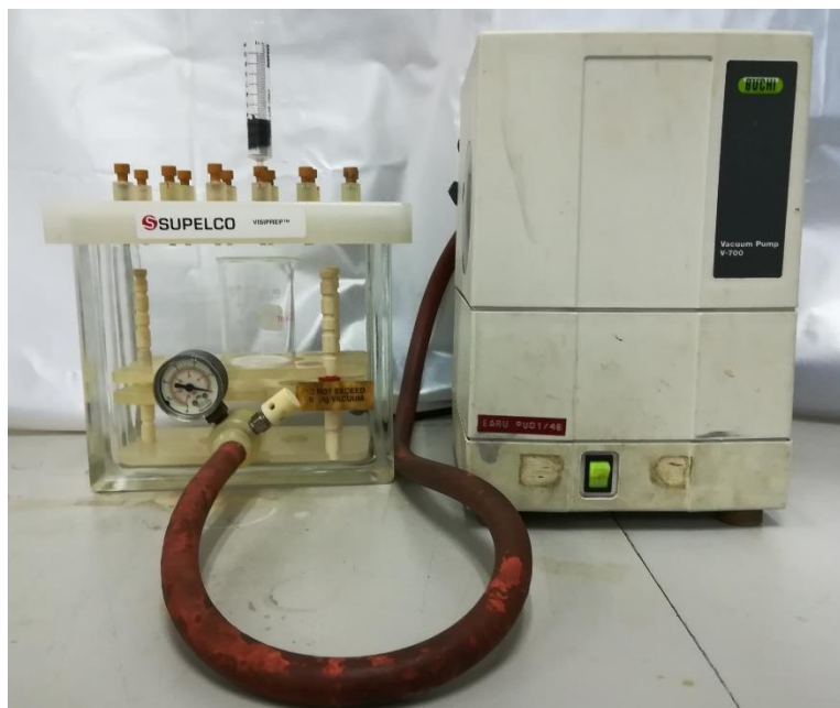
Figure 4.13 Photograph of column system for paraquat removal.
