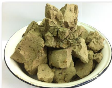
Figure 2.5 Sludge from Metropolitan Waterworks Authority, Bangkok, Thailand.
