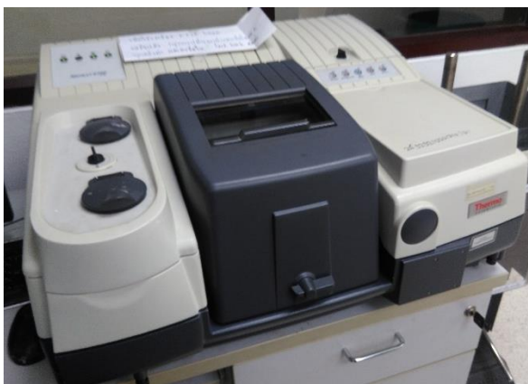
Figure 3.6 Fourier transform infrared spectrometer (Thermo Scientific model Nicolet 6700)
