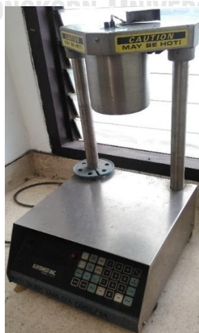
Figure 3.9 Melt flow indexer (model 7053)
