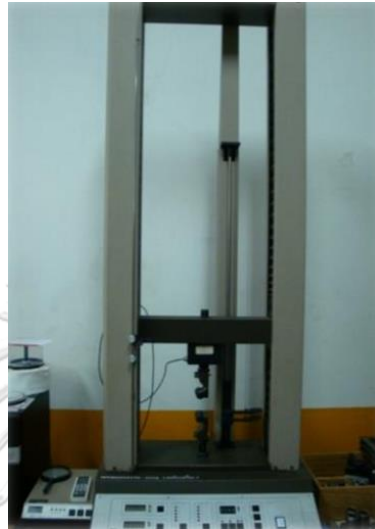
Figure 3.12 Universal testing machine (model H10KM)
