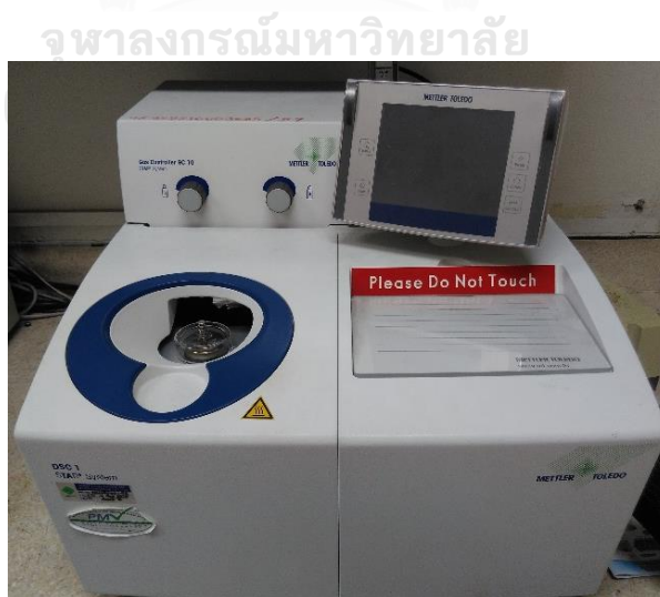
Figure 3.7 Differential scanning calorimeter (Mettler Toledo, DSC 1 STAR System)
