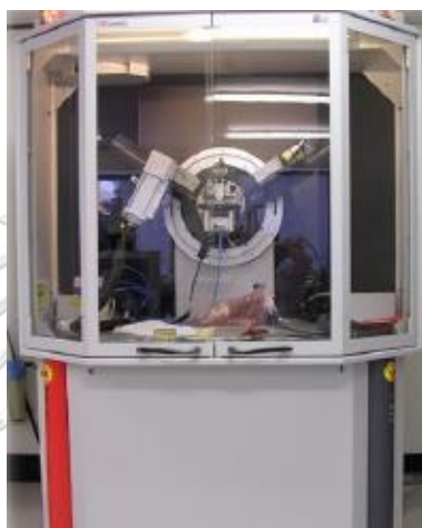
Figure 3.5 X-ray diffractometer (Bruker AXS D8 Advance X-ray diffractometer)
