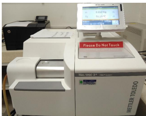
Figure 3.8 Thermogravimetric analyzer (Mettler Toledo, TGA/DSC 3+ STAR System)
