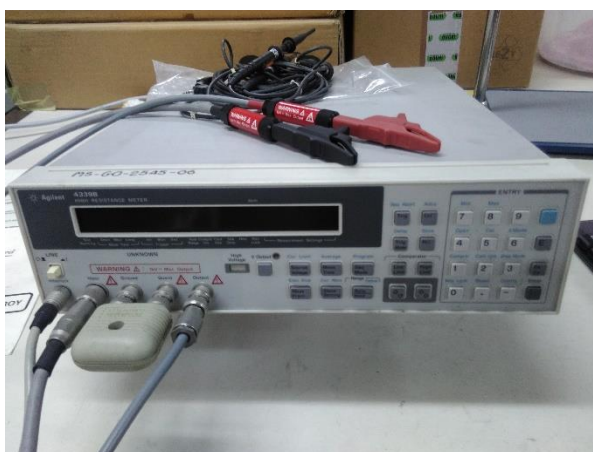
Figure 3.14 High resistance meter (Agilent model 4339B)
