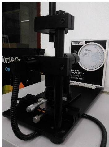
Figure 3.11 Contact angle meter (model CAM-PLUS)
