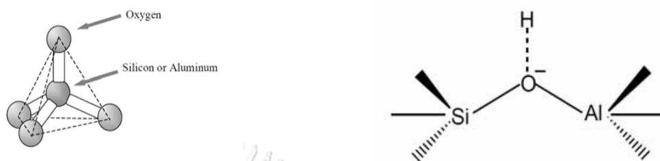
Figure 2.1. Zeolites' primary building unit (Left) and a typical chemical structure of zeolite (Right) [8].
