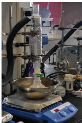
Figure 3.3. Reflux condenser set-up for acid dealumination.
