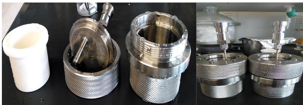
Figure 3.1. Stainless-steel autoclave reactor used in this research work.
