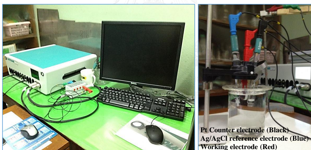
Fig. 2.7 PGSTAT 302N for corrosion testing
