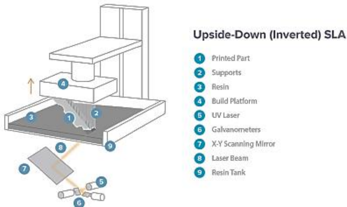
Schematic of the upside-down (Inverted) SLA systems
