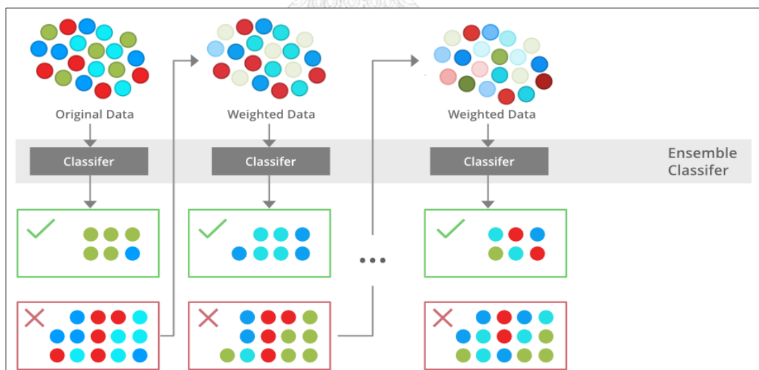
Figure 8 Visualization of XGBoost algorithm [20]
