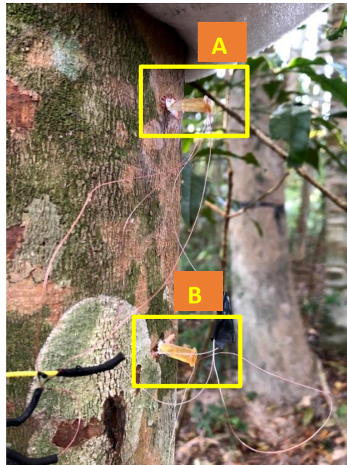
Figure 3.3 Self-constructed thermal dissipation probes (TDPs) contain (A) heated probe and (B) non-heated probe or reference probe.
