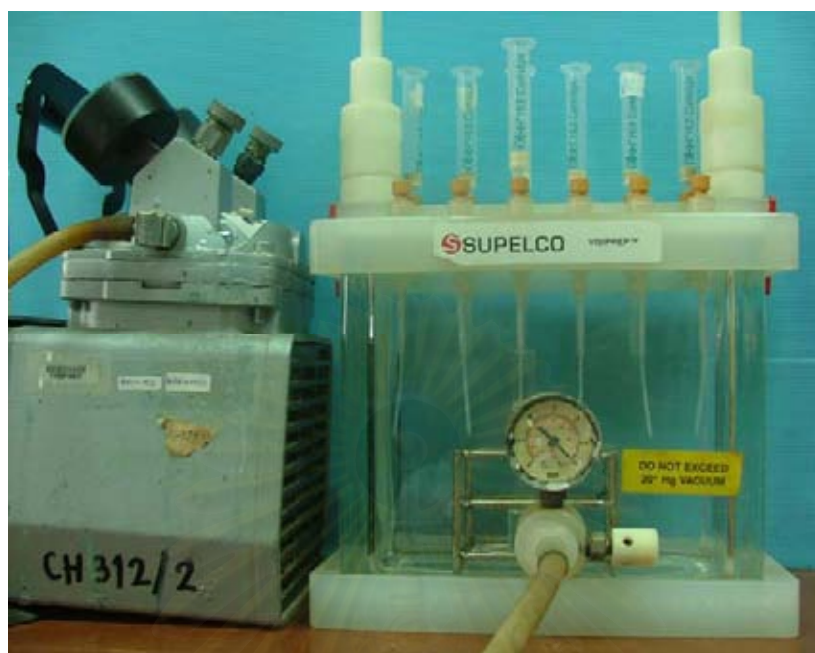
Figure 3.1 SPE Manifold Connected with the Pump
