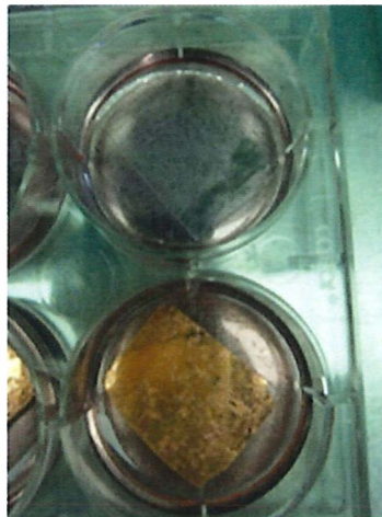
Figure 3. Top well – peeling problem was observed for gold thin-film substrate; bottom well – attachment of film was improved for gold-chromium thin-film substrate
