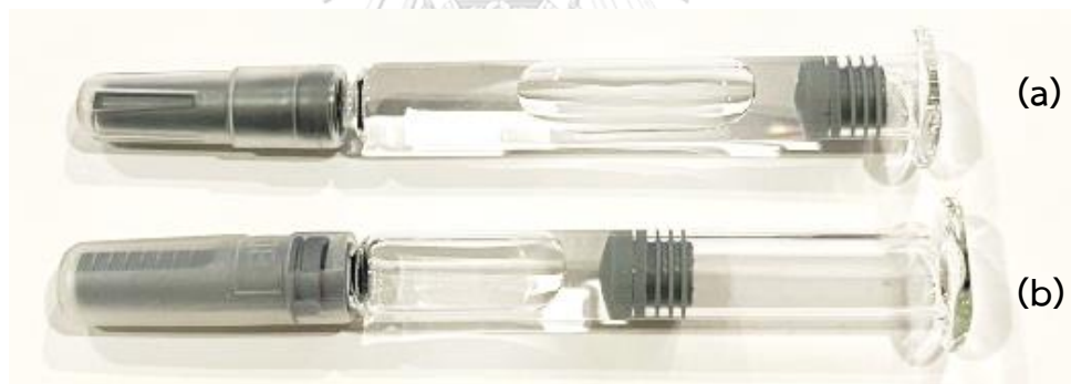
Figure 30 Sample with 0.32 cm 3 head space (a) Filling volume 1 mL (b) Filling volume 0.4 mL
