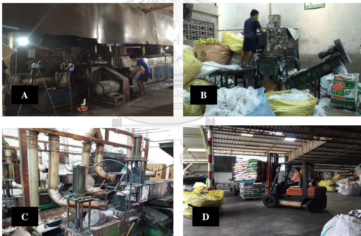
Figure 4.12 Several areas and process inspected under the hazard identification: (A) Extrusion; (B) Shredding; (C) VOCs emission from extruders; (D) Warehouse
