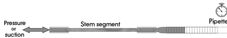
Figure 3.5 Diagram for measuring flow rates through a stem segment 20
