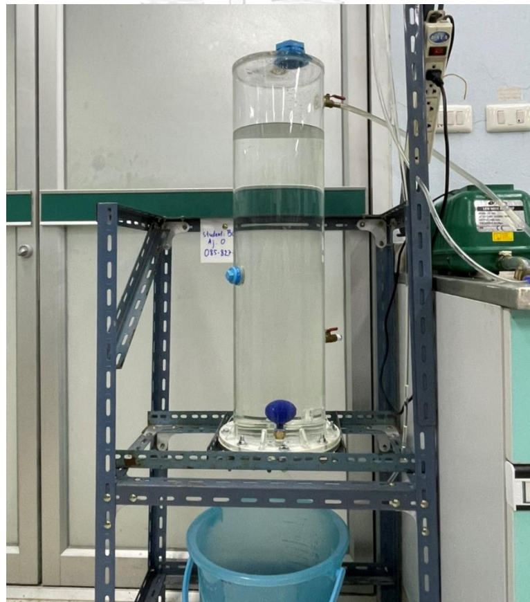
Figure 3.2 Experimental set-up of bubble column reactor (BCR)
