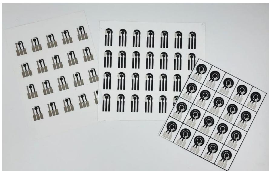
**Figure 2.2** The electrochemical sensors based on polymeric substrate.
