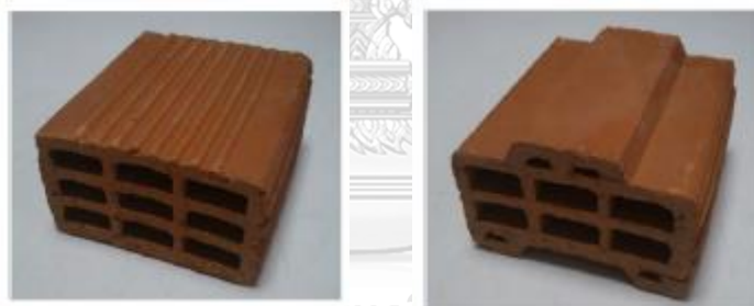
Figure 2.3. Standard brick units and locked brick units
