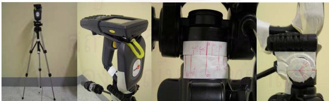
Figure 5.3 From left to right: Portable reader was attached on a tripod, 3D view of portable reader, horizontal scale for horizontal rotation, and vertical scale for vertical rotation
