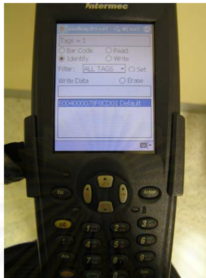
Figure 5.4 The appearance of standard user interface on Intermec 700 Series Color Mobile Computer
