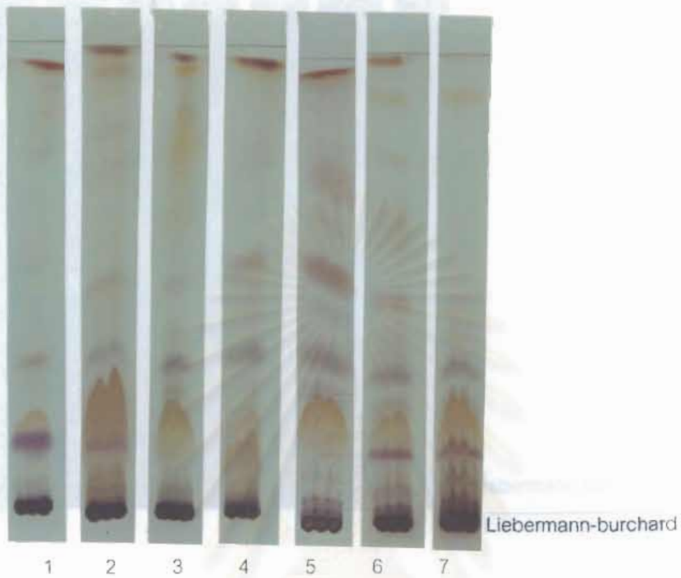
Fig 87 One dimensional TLC patterns of the extracts of Kaysorn-tung-haa, Ma-li-son and Kra-thing flowers dection Liebermann-burchard.
