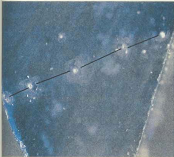
Figure 9: A natural blue sapphire (DIF1), reportedly simply heat-treated, was cut in half and the five points shown where LA-ICP-MS analyses were made (see Figure 10). Photo by P. Lomthong
