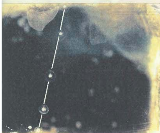
Figure 13: A rectangular block of a natural blue-green sapphire (BG1), heat-treated with Be by a Thai heater, showing surface-related yellow rim surrounding the complex blue core (a, in immersion liquid). After the treatment the sample was cut in half (b, in immersion; c, in air) and analyses were made at five points across the cut surface by LA-ICP-MS. Two points on both rims are very close to the yellow zone (rim) while three points in the middle are only in the blue core. Photos by C. Somboon.
